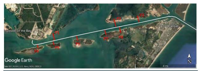
Figure 6.2: Location of the XBEACH profile models (red) along the Port of Corpus Christi Shipping Channel
