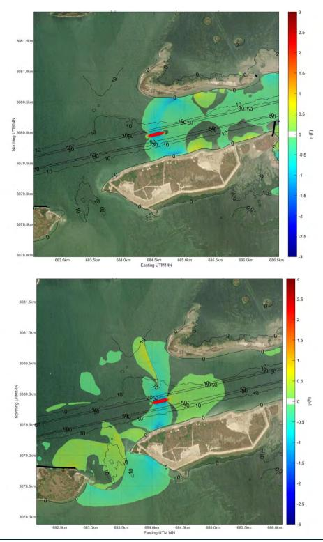
Figure 4.3: Example Primary Wave Field for an Inbound (left) and Outbound (right) Suezmax Vessel (Mean Speed) Scenario (Water Level Surface in ft relative to SWL)
