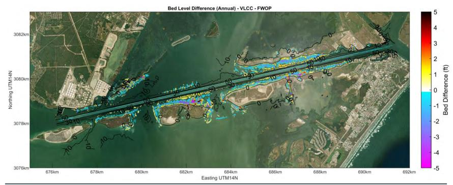
Figure 5.3: Annualized Bed Level Change under Future Without Project Channel Conditions for VLCC vessel traffic
