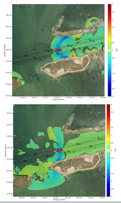
Figure 4.5: Example Primary Wave Field for an Inbound (left) and Outbound (right) VLCC Vessel (Mean Speed) Scenario (Water Level Surface in ft relative to SWL)
