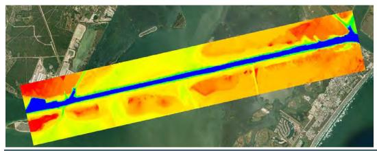
Figure 2.2: Extent of the FUNWAVE domain with color scale based on model depths for the existing channel condition
