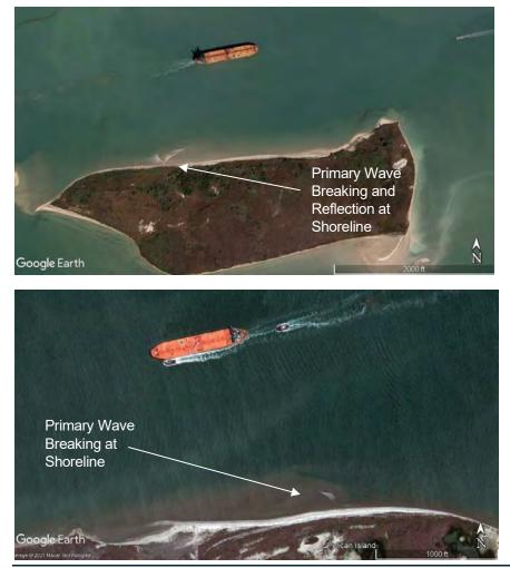
Figure 1.3: Examples of Tanker Generated Primary Waves Breaking along the Shoreline of Corpus Christi Channel
