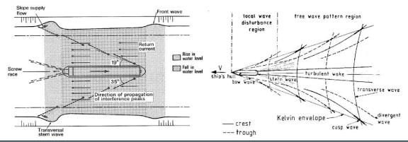
Figure 1.2: Schematics of the Primary (left, from PIANC, 1987) and Secondary (right, from CRISP, 2001) Waves Induced by Ship Motion
