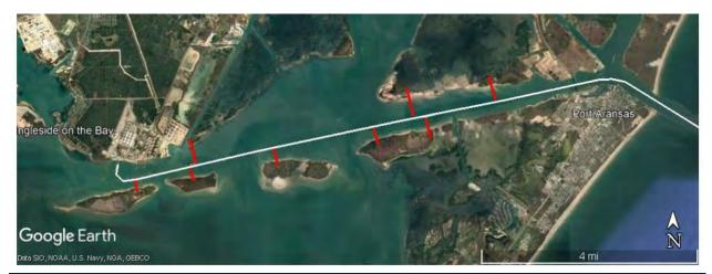
Figure 2.3: Location of the XBEACH profile models (red) along the Port of Corpus Christi Channel
