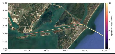
Figure 3.4: Tracks and speed profiles of outbound transits from the Ingleside terminal from AIS data for VLCCs and Suezmaxs (2019 – 2020)
