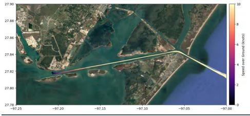
Figure 3.3: Tracks and speed profiles of inbound transits to the Ingleside terminal from AIS data for VLCCs and Suezmaxs (2019 – 2020)
