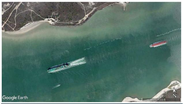
Figure 1.4: Example of Tanker Generated Secondary Waves in the Corpus Christi Channel
